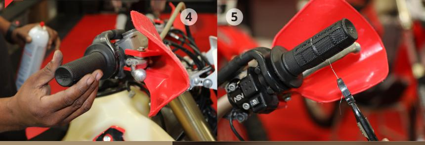
4 > After glue is added to the new throttle, Holly sprays some silicone lube into the new rubber handle and slips it over the throttle
