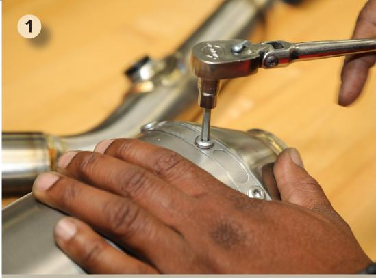
**1** > Holly adds a red thread sealer to all bolts that are attached to the exhaust system to keep them from shaking loose.
